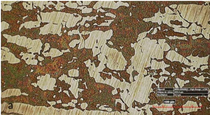
Figure 3. Microstructural recovery, a: heat-treated at 750°C for 1hr, b: heat-treated at 1050°C for 1hr (both air-cooled).
