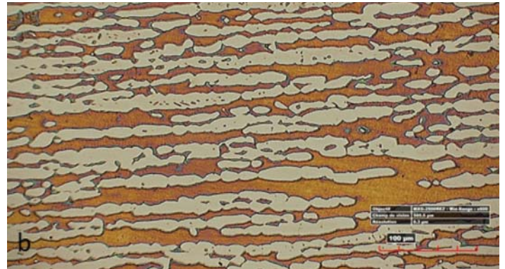
Figure 3. Microstructural recovery, a: heat-treated at 750°C for 1hr, b: heat-treated at 1050°C for 1hr (both air-cooled).
