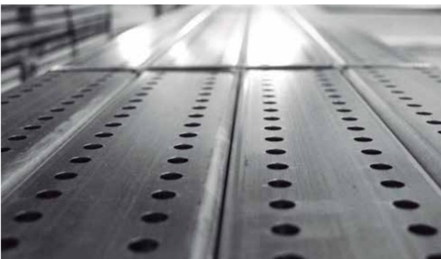
Laser cutting is one of the services whereby Stalutube enables its clients to customize the products according to their needs.
